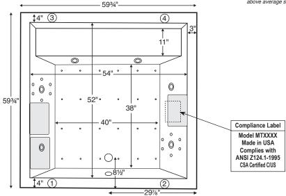
Numbered areas on tub deck represent possible locations to install cleaning systems, faucets and other fixtures.
